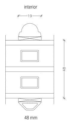
19 mm glazing bars are supplied as standard with a spacer between the glass panes.
