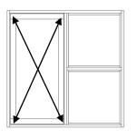
When the frame is fastened, take a cross measurement. Both measurements must be the same.
